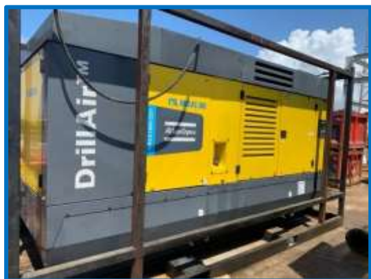
1,600-CFM Air Compressor
