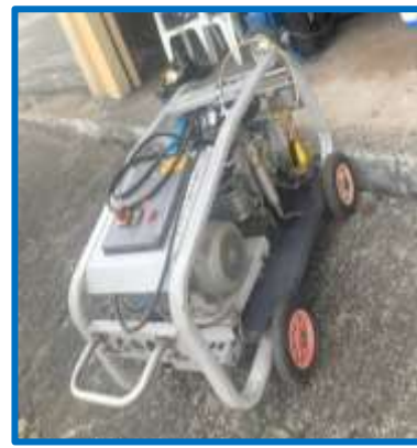
Breathing Air Generator
