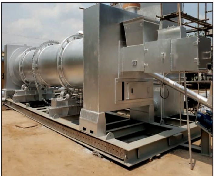
High-Temp Incinerators & LTDUs are used for Oily Waste Recycling & Oil Recovery
